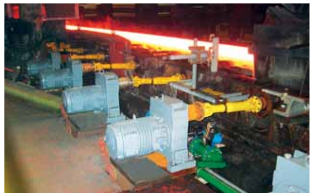
Fig. 6: Delay table with S141-1A ARG 160L 4, M_{\max}=1039 Nm
