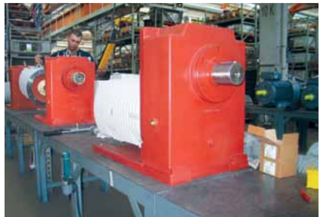
Fig. 5: Roller table version, SG200 ARG 200L 8, M_{\max}=1655 Nm
