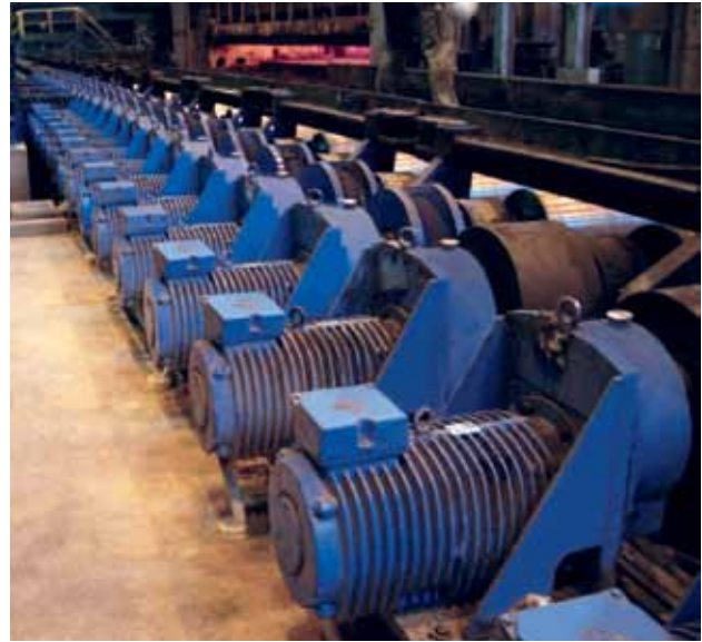
Fig. 4: Furnace table with ARG 200L 12, M_{\max}=1888 Nm
